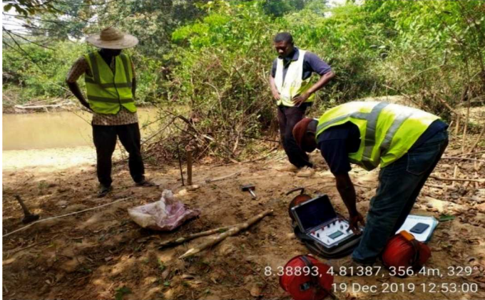
Fig. 2: Conduction of VES and Trial pit for soil sampling at Dugbe-Osin area
