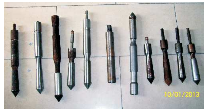
Fig. 5: Some locally fabricated Single and double Cones
