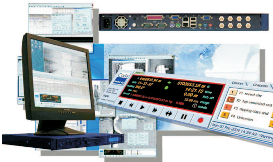
CODA Geophysical Acquisition System
