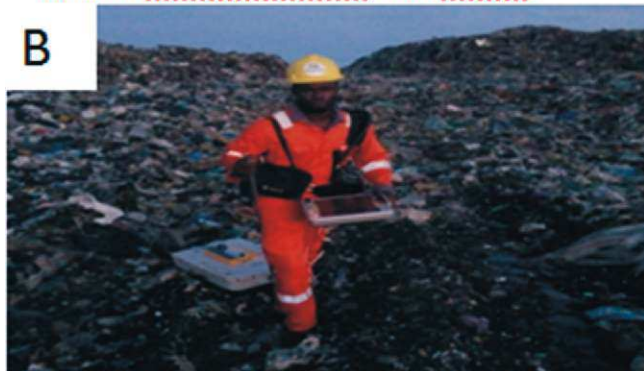
GeoterraIn Intern Acquiring GPR Data using e-tracking along a traverse line in Igando Dump site , Lagos State
