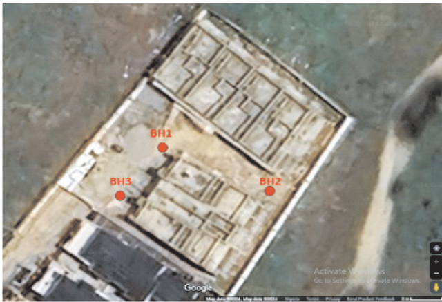
Fig. 4: Distressed building on pile foundation (under construction) and distribution of boring test (Site B).
